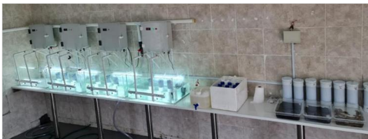
Figure 2. The hatchery at POC with spools in cultivation tanks, and trays with kelp blades in front of canisters (Photo credit: Dr L Botes)
