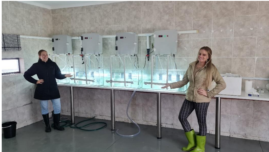
Figure 4. POC based hatchery after set-up with the 1st batch of kelp spools (Photo credit: Dr L Botes)
