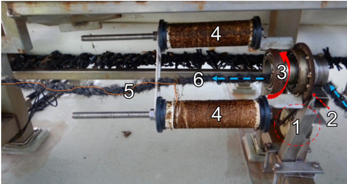
Figure 17. Seeded twine deployed onto grow lines (polypropylene mussel rope) spinning the spools around the rope with the help of a modified electric motor. (1) An electric motor (dashed red circle) that drives (2) a belt (dashed red arrow) and spins (3) two (4) seeded spools around the grow line, thereby winding (5) the seeded twine (orange line) around (6) the grow line (dashed blue arrows) that is subsequently deployed at sea. This method was used in Biancacci et al. (2022c).
