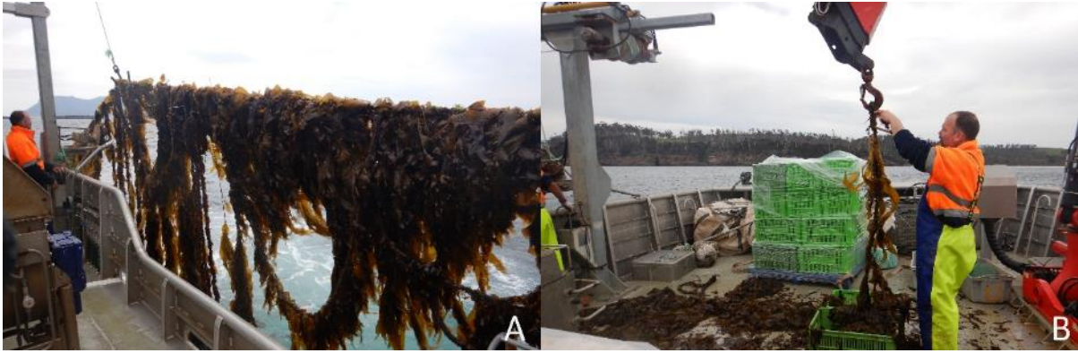
Figure 20. Harvesting of kelp biomass using a repurposed mussel harvesting vessel at Okehampton Bay, Tasmania, in September 2020. (A) The mussel boat geared to anchor and lift the seeded lines deployed in a looped arrangement, and (B) harvesting the biomass manually by cutting the seaweeds from the cultivation lines.
