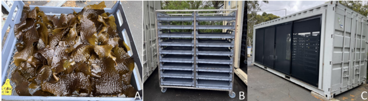
Figure 24. (A) A tray with washed E. radiata biomass harvested in October 2022 ready to be loaded in the dryer, (B) an example of a trolley with 18 trays custom made for the dryer, and (C) an example of the custom-made drip-dry container with mesh doors on either side.
